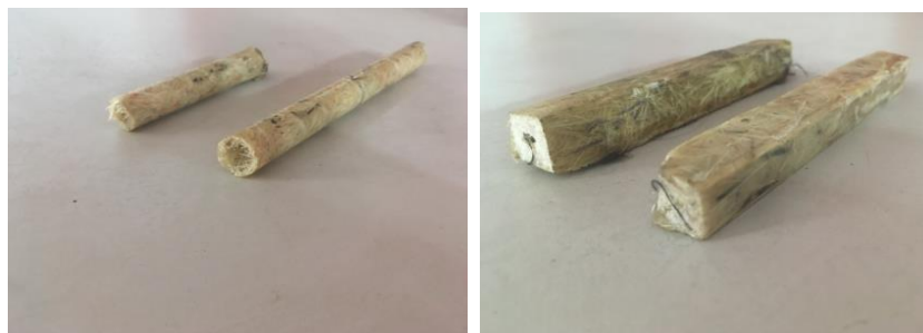
Fig 6: Specimens of Sisal Fiber Composites for Tensile and Impact Energy Test
